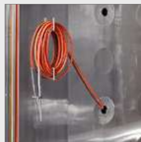
RTD (Resistance Temperature Detectors) temperature probes.
